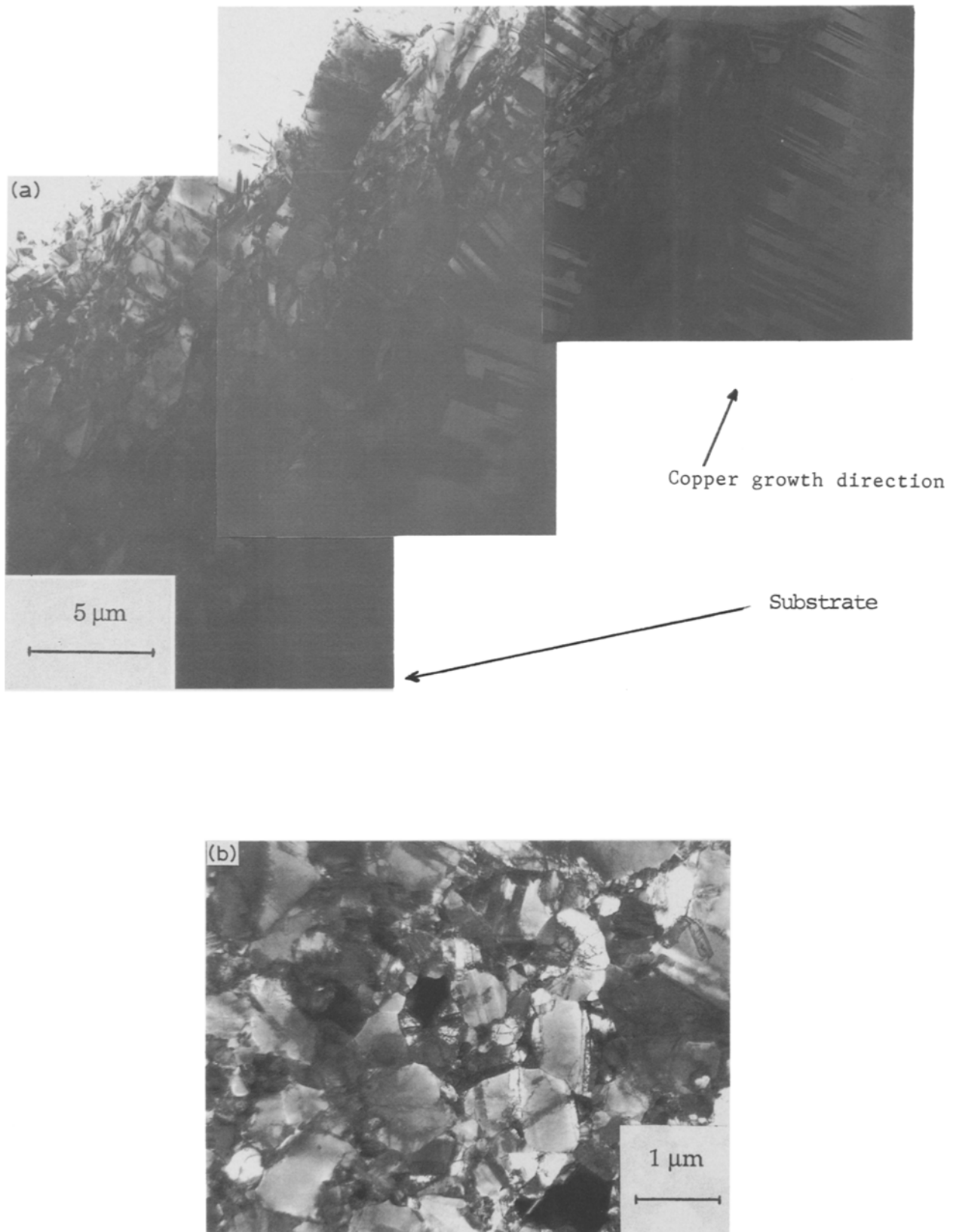
Fig. 7. TEM observation of a (111) FT-UD copper deposit on polished titanium. (a) Section perpendicular to the substrate and (b) section parallel to the substrate.
